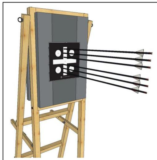
The adjustment to be done here is to move the arrow rest, either to the left or to the right, again in small increments of appr. 1/32" (0,8 mm) each time. If the arrow groups are widening, go back to the original position and adjust the arrow rest in the other direction. If the arrows are lining up along a straight horizontal line, the adjustment is correct.
